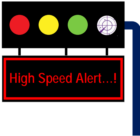
Fig.1. Vehicle Activated Signs (VAS) with Radar embedded, and Vehicle Message System (VMS) message board.
